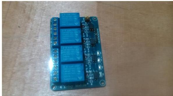
**Gambar 2.5** Relay 4 Channel
