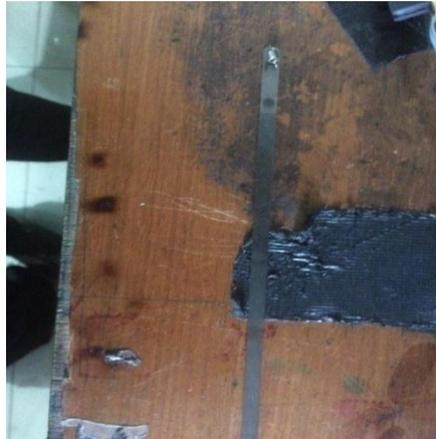
**Gambar 2.7.** *Encoder Panjang Printer Canon ip2770*
