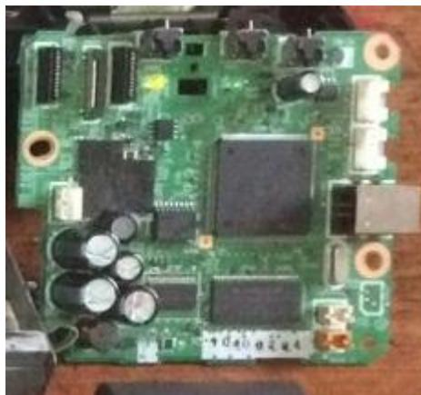
**Gambar 2.11.** *Motherboard* Printer Canon ip2770
