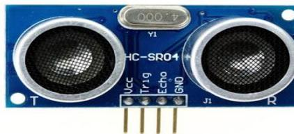
**Gambar 2.4** Sensor Ultrasonik
