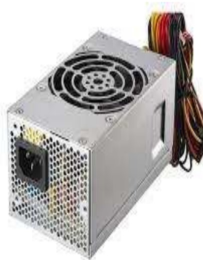
Gambar 2. 6 Power Supply Sumber : (Alexander et al., 2019)
