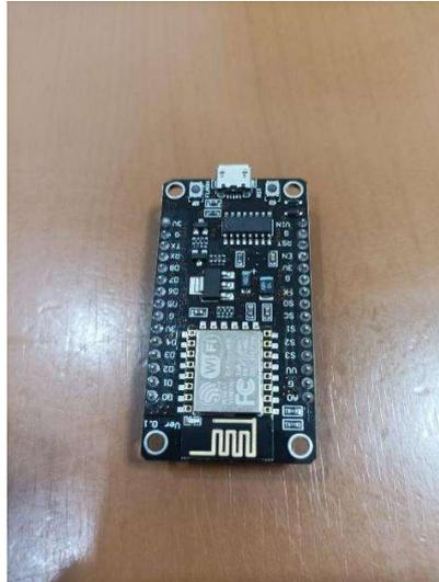
**Gambar 2.1** NodeMCU V3 CH340
