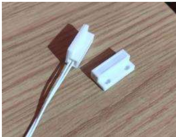
Gambar 2.3 Sensor Reed Switch Sumber : Data Peneliti, 2022
