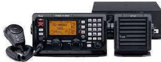
**Gambar 2. 13 SSB (Single-Side Band Radio)**
