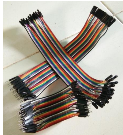
Gambar 2.6 Kabel Jumper Sumber : (Data Penelitian, 2020)
