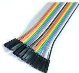
**Gambar 2. 5 Kabel Jumper**
