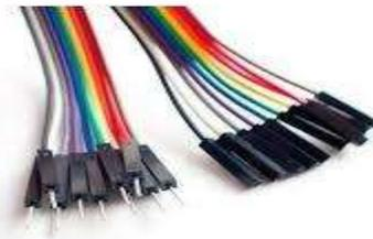
**Gambar 2.10** Kabel Jumper
