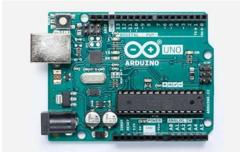
**Gambar 2.1** Arduino Uno Rev3
