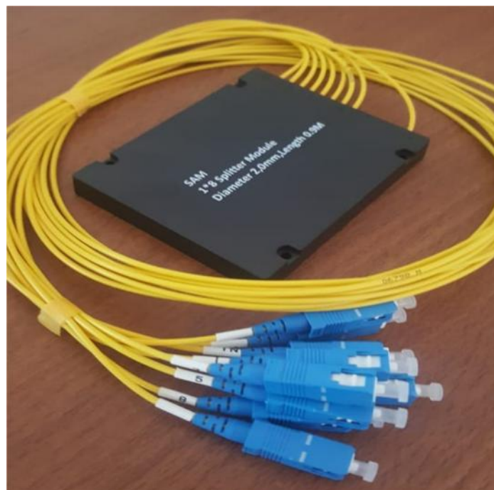
Gambar 2.23 Passive Splitter 1:8 (Sumber: Data Penelitian, 2020)
