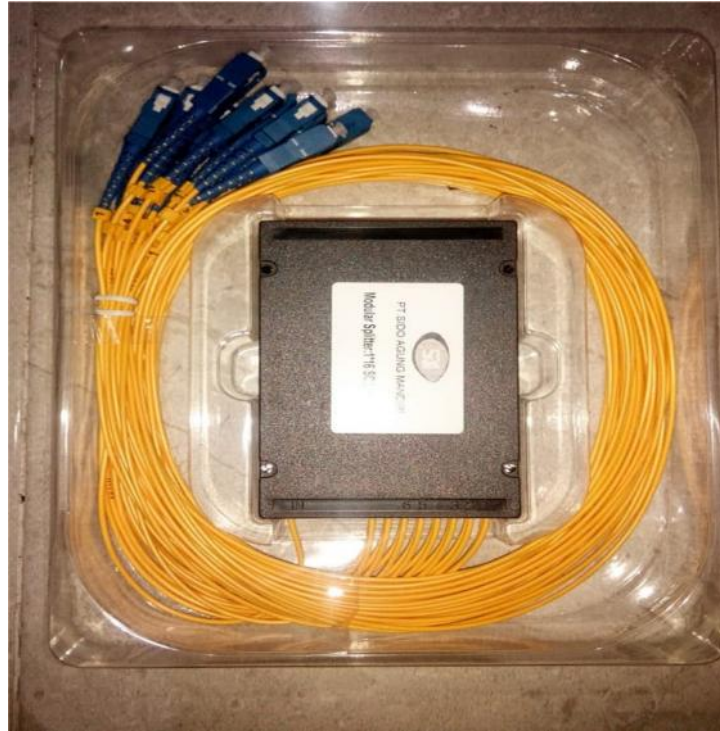
Gambar 2.24 Passive Splitter 1:16 (Sumber: Data Penelitian, 2020)
