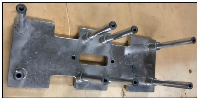
Gambar 2.7 Block Jig Lifter
