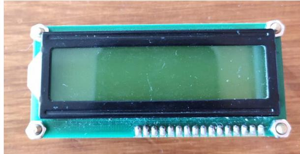
**Gambar 2.11** *LCD Display*
