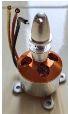
**Gambar 2.8** *BLDC Motor A2212/10T 1400KV*
