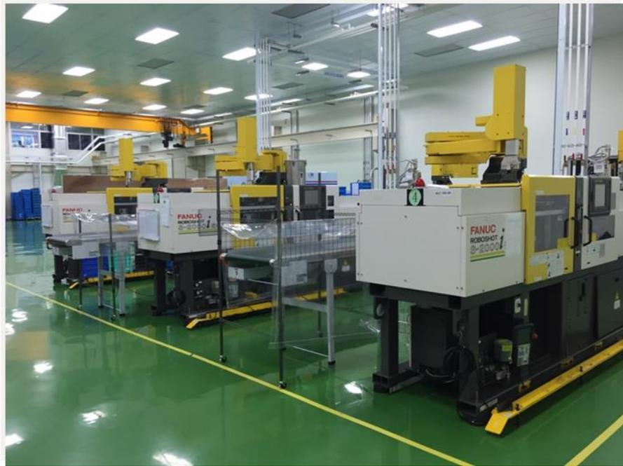
**Gambar 2.2** Mesin *Injection Molding FANUC S-150T*
