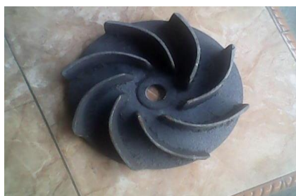
Gambar 2.11 Impeller (data penelitian 2019)
