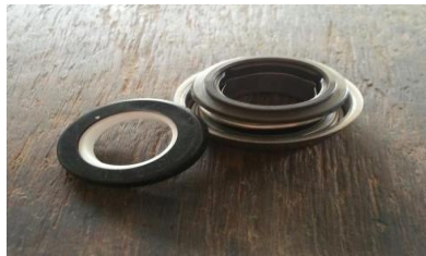
Gambar 2.13 Seal Pompa (data penelitian 2019)
