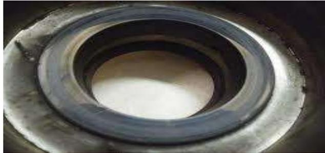
**Gambar 2.5** *Mechanical Seal*
