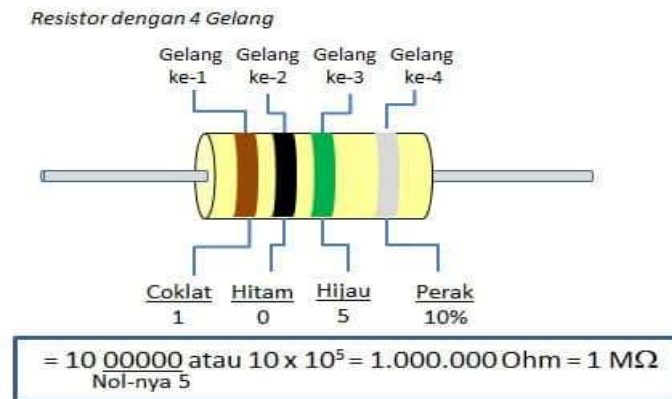
Gambar 2.12 Membaca Nilai Gelang Resistor .
