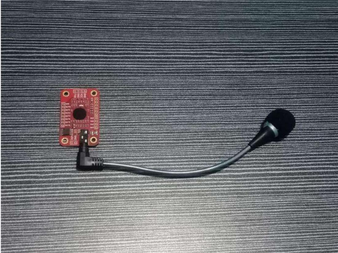
**Gambar 2.5.** Module Voice Recognition V3
