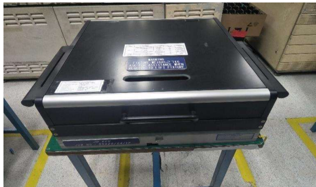
Gambar 2. 6 Fixture ICT ( In Circuit Test )
